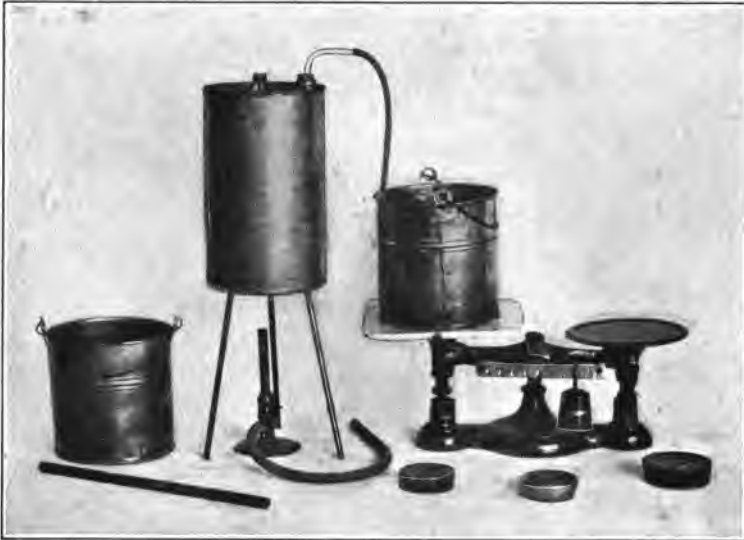
FIG. 21. Apparatus used to show that equal weights of steam and boiling water at the same temperature have different heating effects.
